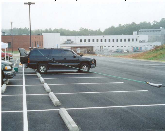
FT- 897 connected to 59' NVIS 75m antenna Suburban is used as counterpoise (huge ground)
