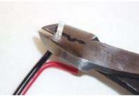
This is the first crimp of a PowerPole 30 amp pin. Notice it is in the first die #1 with #12 wire and that the seam in the pin is against the rounded side of the tool's die. Make sure the end of the pin's crimp section is just below flush on the side of the tool.
