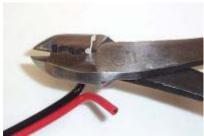
This is the 2nd step of a PowerPole 30 amp pin. Notice that the pin is in the back die # 3 and is turned 90degrees. Do not crimp this very much, just enough to make the width of the crimped section less that what it was before you started. Again make sure the end of the pin's crimp section is just below flush on the side of the tool.
